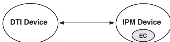
Figure 11. T1/E1 Gateway Example
