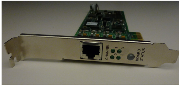
Figure 4. End Panel RJ 45 Connector and LEDs
