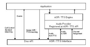
The above figure shows the overall architecture. The streaming part of the ASR / TTS engine registers to the Dialogic<sup>®</sup> Diva<sup>®</sup> SDK via the so called "Audio Provider Interface". The application uses the standard registration at the Diva API.
