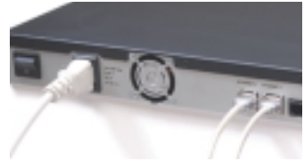
Rear-view of a unit, showing LAN ports, power outlet and on/off switch
