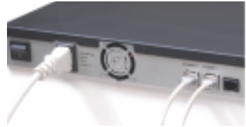
Rear-view of a unit, showing Ethernet ports, power outlet and on/off switch
