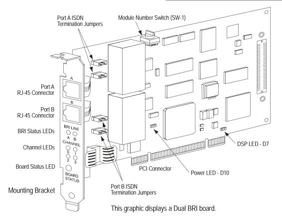
Figure 5. Dialogic® Brooktrout® TR1034 BRI PCI Series Fax Board
