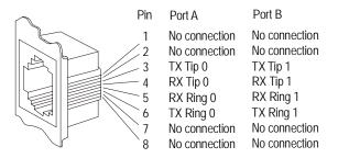
Figure 4. Connector Pinouts
