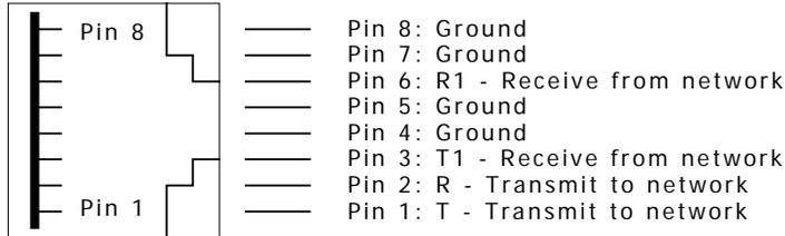
Pins 4, 5, 7, and 8 are grounded through a spark gap for 100Base-T Ethernet connections
