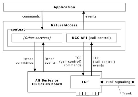
CAS API software provides a series TCPs for a variety of protocols. The TCP is loaded into the on-board memory of a line interface board when you configure the board. For applications that must support multiple protocols and/or protocol variations simultaneously, more than one TCP can be loaded to the telephony board at the same time. Each line supports one TCP at a time.
