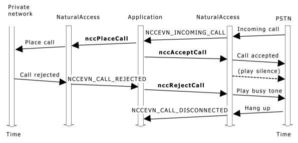
The way a gateway application rejects calls is similar to the way it accepts calls. Initially, the TCP accepts the incoming call and puts it on hold by sending silence to the line. When the outbound call is rejected, the application calls **nccRejectCall**. The TCP immediately starts to perform the action requested by **nccRejectCall**. It can play a busy tone, or let the application play a reject message. The TCP then relies on the caller side to tear down the connection.
