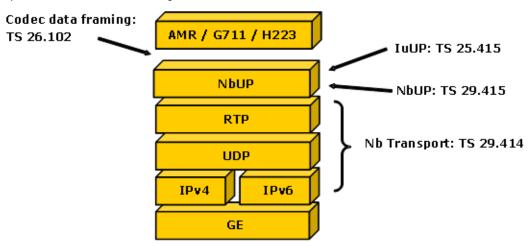
The NbUP protocol (TS 29.415) is almost identical to the Iu UP protocol (TS 25.415). Because the NbUP uses the same PDU types as the Iu UP, the term IuFP is used to refer to the common framing.
