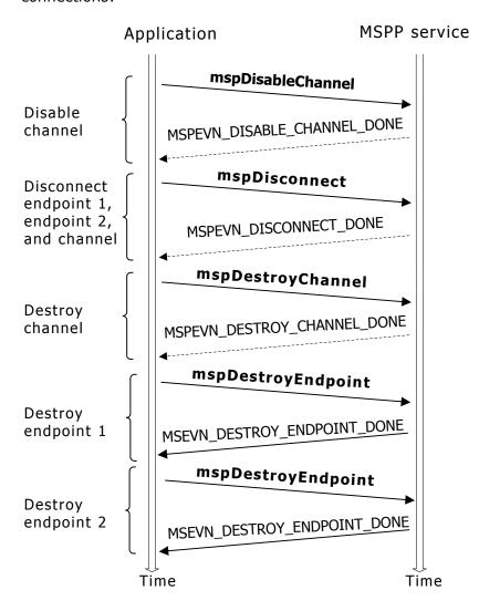
Applications can interrupt a connection either by disabling the channel with **mspDisableChannel**, or by disabling one of its component connection endpoints with **mspDisableEndpoint**.
