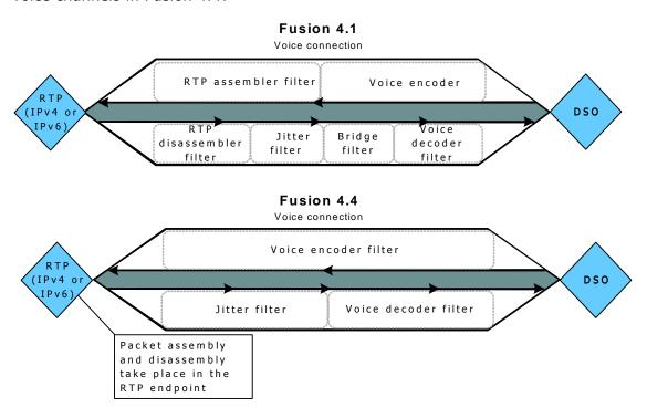
In Fusion 4.4, simplex voice connections, either the voice decoder or voice encoder filter is omitted from the voice channel (depending on the direction of the data transfer). The following illustration shows the difference between T.38 fax connections in Fusion 4.1 and Fusion 4.4:
