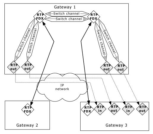
In this configuration, RTP out endpoints on Gateway 1 act as monitoring endpoints that direct intercepted voice data to Gateway 3.
