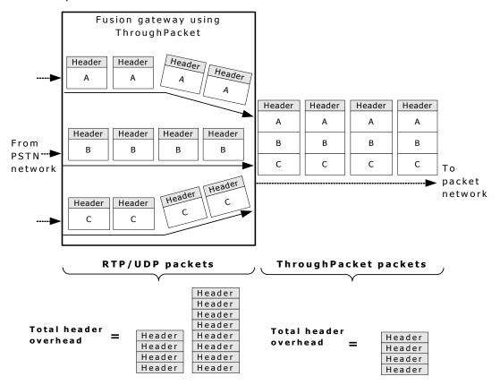
ThroughPacket's enhanced efficiency in transferring data reduces the total bandwidth the application needs to transfer voice data across the network. By multiplexing many streams of RTP data, a VoIP system employing ThroughPacket technology is able to provide two major benefits:
