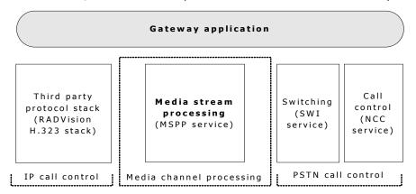
In both models, application initialization, PSTN call control, and switching are controlled by Natural Access and its services (ADI, NCC, and SWI services). Call control at the IP network interface can be performed through a third party protocol stack such as the SIP or H.323.
