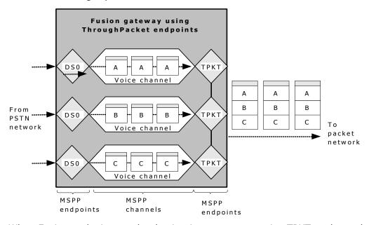
When Fusion endpoints at the destination gateway receive TPKT packets, they demultiplex the data and direct the individual payloads to their separate destinations.
