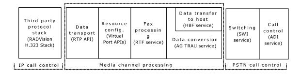
The following illustration shows the simplified Fusion 4 programming model. Notice that all of the media processing tasks, formerly performed with several different APIs and services, are now accomplished with the MSPP service only:
