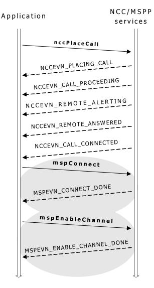
The following illustration shows the call setup function sequence as the application monitors call progress from the time the MSPP connection is initiated until the call is answered:
