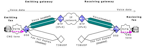
When a calling fax machine sends a CNG tone (indicating that a fax terminal is calling), the tone is carried across the network as voice data. The called fax machine responds by sending a CED tone.
