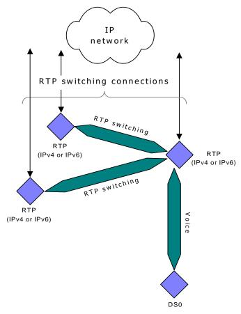
Fusion RTP switching channels consist of a single switch filter used to transfer data between separate RTP endpoints. When applications use an RTP switching channel to connect the two RTP endpoints, the channel transfers the voice packets received on one RTP endpoint to the other RTP endpoint without performing any data conversion tasks.
