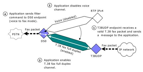
The following illustration shows the emitting and receiving gateways transferring fax data after voice/fax switchover has taken place:
