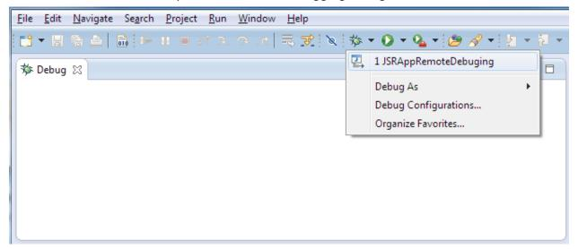
Once the **remote debugging configuration** is selected and a connection is established, the content of the **Debug** window should show running threads. The Eclipse project is connected to the build application that is deployed in TeleStax Application Server.
