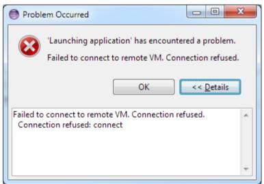
4. Open the **Debug** perspective in Eclipse (**Windows** > **Open Perspective** > **Debug**). If nothing appears in the **Debug** section, then a connection to the Application Server has not been established. To connect/reconnect, go to the debug icon on the toolbar and choose the newly created remote debugging configuration.
