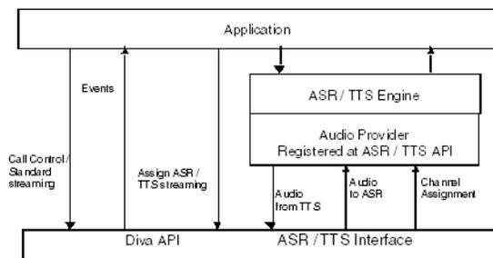
The above figure shows the overall architecture. The streaming part of the ASR / TTS engine registers to the Dialogic® Diva® SDK via the so called "Audio Provider Interface". The application uses the standard registration at the Diva API.
