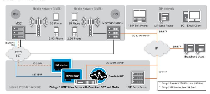
Figure 4. 3G-324M Video with Dialogic® PowerMedia™ HMP for Linux (HMP Linux)
