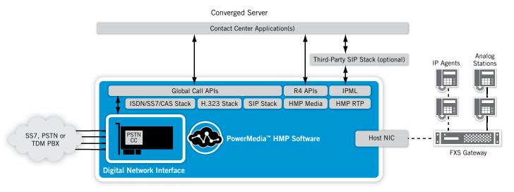
Figure 2. Converged IP Contact Center Architecture
