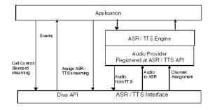
The above figure shows the overall architecture. The streaming part of the ASR / TTS engine registers to the  $Dialogic^{(\!R)}$   $Diva^{(\!R)}$  SDK via the so called "Audio Provider Interface". The application uses the standard registration at the Diva API.
