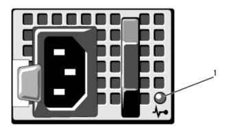
The power supply status indicator lights up as follows to show power supply conditions:
