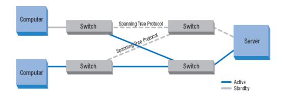
ANS provides fault tolerance for different network architectures, with both single and multiple switch connections supported.
