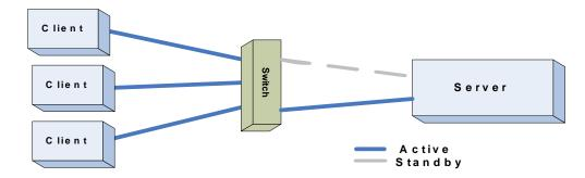
Switch Fault Tolerance, in contrast, supports a failover relationship between two adapters when each adapter is connected to a separate switch. In SFT, if one adapter, its cabling or the switch fails, the other adapter takes over, as in the following diagram.
