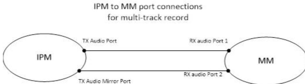
This use case makes use of “mirrored” port that mirrors the data coming into the RX port of an IPM device. This RX data is what will be sent out over the IP network. The “tx mirror” port mirrors the data from the RX side back into a TX port for transmission to other HMP components.
