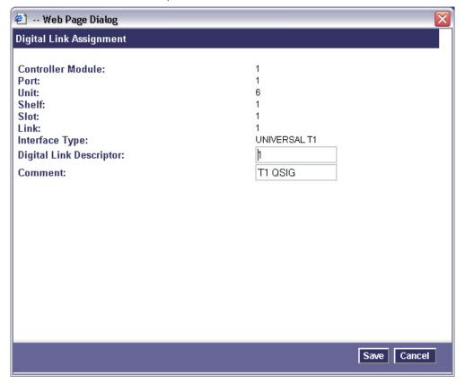
Use the ISDN-PRI MSDN-DPNSS-DASSII Trunk Circuit Descriptor menu selection to assign direction and protocols to the individual trunk cards in the PBX.
