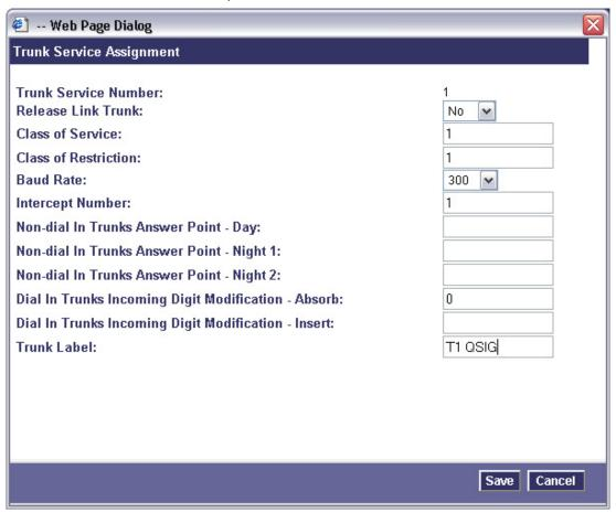
Use the ISDN-PRI Digital Trunk Assignment menu selection to configure the individual trunk members and assign them the defined Trunk Service Assignment template and Trunk Circuit Descriptor template that were configured in the previous steps. This gets done for each member of a trunk interface.
