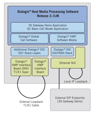
Figure 1. High-Level Architecture
