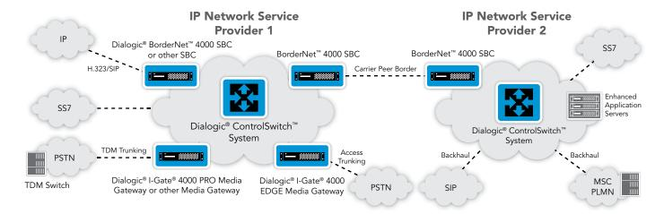
Figure 1. Multi-Service Dialogic® ControlSwitch™ System Deployment
