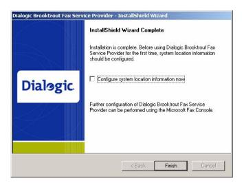
15. The screen above indicates the successful Brooktrout FSP installation. You can select the checkbox if you want to configure the system location information which launches a Microsoft telephony configuration utility. Click **Finish** to exit.
