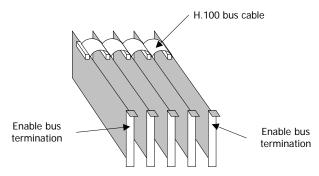
DIP switch S2 on the TX 4000 board controls the H.100 bus termination. By default, all S2 switches are set to the OFF position. H.100 bus termination is disabled. To enable H.100 bus termination, set all S2 switches to the ON position only for the boards that are on the ends of the H.100 bus.
