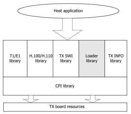
After a system reset, the TX boards are left in a reset state. TX-based system and protocol tasks must be downloaded to the TX board memory. Refer to the *Task executable list* on page 10 for more information. TX-based tasks are usually downloaded with the *cplot* utility, which uses the Loader library to load tasks to the TX board. The Loader library enables you to develop custom applications that perform task loading with an interface rather than by calling the *cplot* utility.
