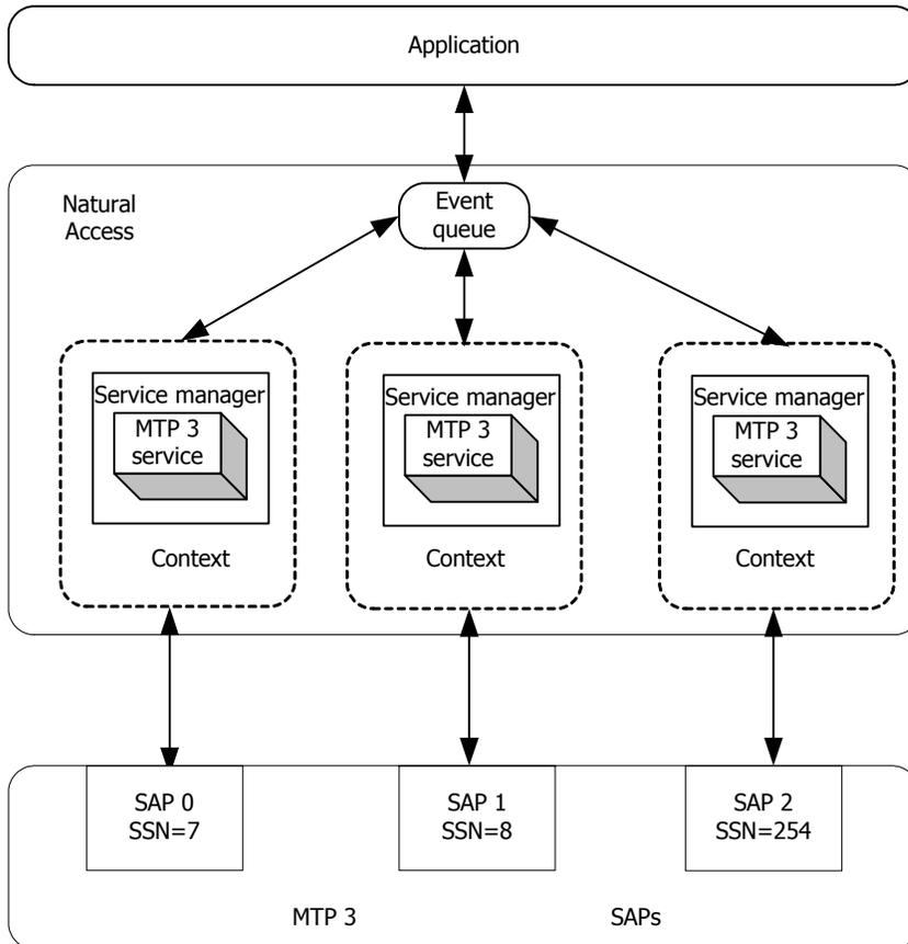
For multi-threaded applications using multiple MTP 3 SAPs (one per thread), a multiple context, multiple queue model is recommended. Each thread has its own independent event loop, receiving only the events associated with its MTP 3 SAP on its Natural Access queue.
