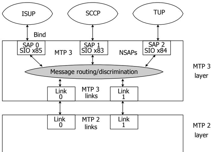
If multiple protocol variants are configured on the same MTP 3 instance (same board), two SAPs are required for each application: one for each protocol variant. In this case, a single application can associate itself with both SAPs for that service, or separate applications can be used for each protocol variant.
