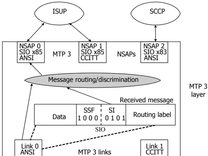
Only the link type of the incoming link and the service indicator portion of the SIO (service information octet) in the incoming message are used to choose the NSAP to receive the incoming message; the sub-service field of the SIO octet (national/international indicator and optional message priority) is not used.
