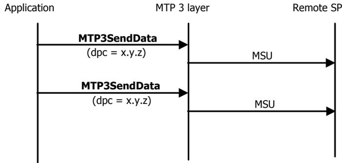
Asynchronous notification and polling are two methods for an application to receive incoming data or status indications. Polling requires the application to call **MTP3RetrieveMessage** to continually check for incoming messages. The application must call this function regularly to avoid excessive queuing of messages in the TX driver or the MTP 3 task. **MTP3RetrieveMessage** returns MTP3\_NO\_MSG until a message is available. It returns MTP3\_SUCCESS when a message is available.
