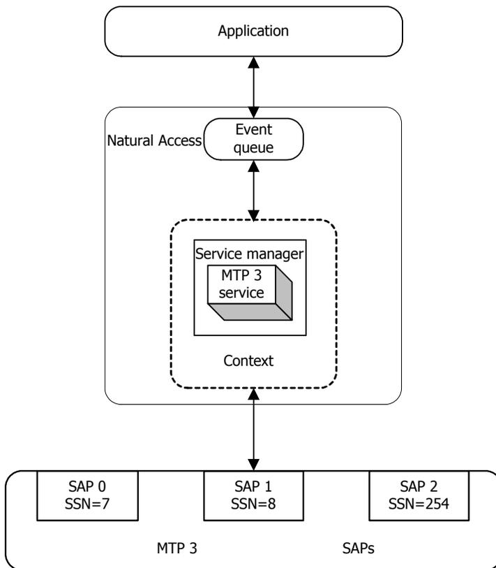
For a single threaded application that uses multiple MTP 3 SAPs (multiple MTP 3 subsystems), a multiple context, single queue model is recommended. The application has a single event loop with events from all SAPs delivered through the same queue. The application determines which SAP a particular event is associated with from a service user ID (suID) value returned with each event.
