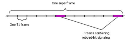
With ESF framing, an extra bit appears after every frame, as in D4 framing. However, only every fourth extra bit is used for framing. This bit is set or reset in a pattern that repeats once every 24 frames, instead of the 12-frame repetition in D4 framing. The 24 frames in the cycle constitute one extended superframe.
