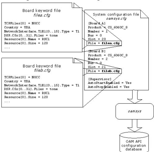
When you run *oamsys*, it creates OAM database records based on the contents of the specified system configuration file and board keyword files. It then directs the OAM API to start the boards, configured as specified.
