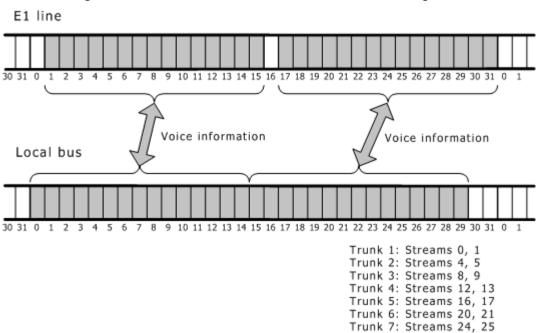
The following illustration shows how voice channel data is assigned to timeslots:
