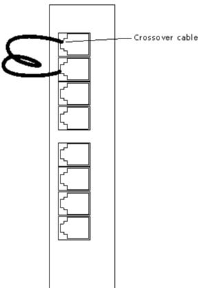
The crossover cable connects the transmit signals from one trunk to the receive signals on another trunk by connecting the pins.
