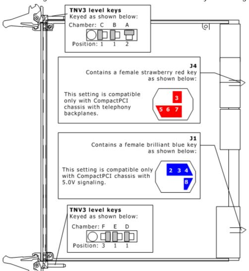
The following illustration shows how the CG 6060C board keys are configured:
