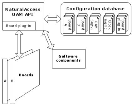
Each OAM API database parameter and value is expressed as a keyword name and value pair (for example, Clocking.HBus.ClockMode = MASTER\_A). You can query the OAM API database for keyword values in any component. Keywords and values can be added, modified, or deleted.
