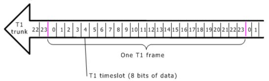
The CG 6060C board supports two T1 framing formats: D4 framing and extended superframe (ESF).
