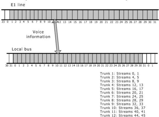
The following illustration shows how voice channel data is assigned to timeslots:
