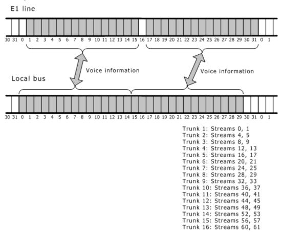
If NetworkInterface.T1E1[x].SignalingType = CAS (the default setting), signaling information is routed to accommodate channel associated signaling. Line channel 16 carries the signaling information for all channels.
