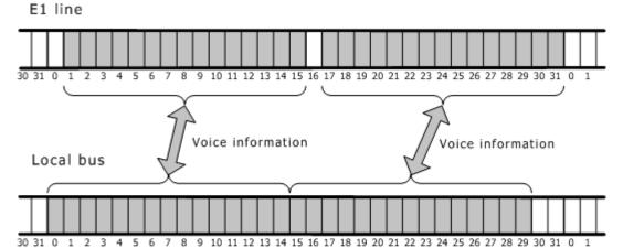
Trunk 1: Streams 0, 1 Trunk 2: Streams 4, 5 Trunk 3: Streams 8, 9 Trunk 4: Streams 12, 13 Trunk 5: Streams 16, 17 Trunk 6: Streams 20, 21 Trunk 7: Streams 24, 25 Trunk 8: Streams 28, 29
