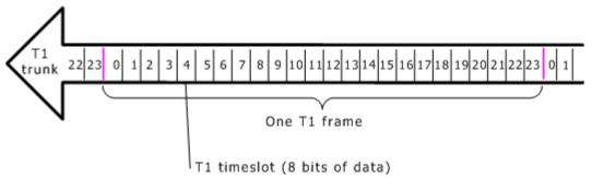
The CG 6565E board supports two T1 framing formats: D4 framing and extended superframe (ESF).
