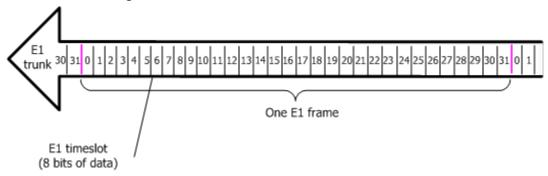
In each frame, channels are numbered 0 through 31. Half of the first channel (channel 0) is used for frame synchronization. The other half can be used as a facilities data link (FDL).
