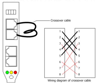
The crossover cable connects the transmit signals from one trunk to the receive signals on another trunk as shown.
