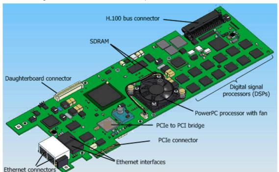
The following illustration shows where components are located on a CG 6565E board:
