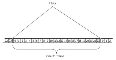
After each frame, the F bit is set or reset according to a pattern that repeats once every 12 frames: 100011011100. This makes the F bit recognizable even in the high-speed T1 bit stream. The 12 frames in this cycle constitute one superframe.
