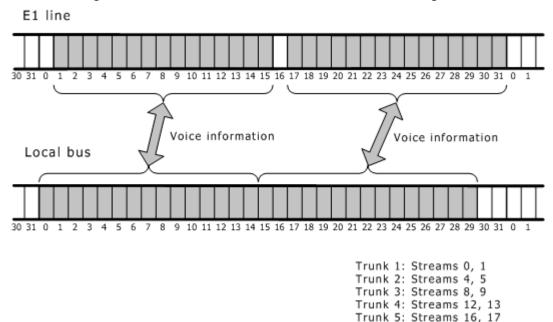
The following illustration shows how voice channel data is assigned to timeslots:
