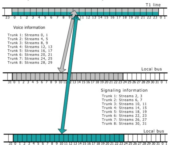
The following illustration shows how data is assigned to timeslots on a T1 trunk:
