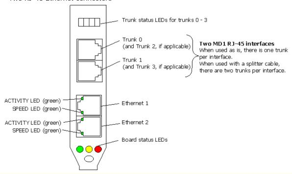
**Note:** CG 6565E boards configured to support one- or two-trunks use an MD1 RJ-45 interface wired as RJ-48C connector.
