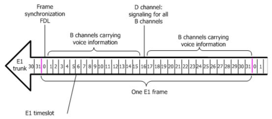
With CAS protocols, four ABCD bits are sent for each channel at a time. Since timeslot 16 can carry only 8 bits of information per frame, it is not possible to send the signaling for all 30 channels in each frame. Therefore, channels take turns using channel 16, two at a time. It takes 15 frames to cycle through the signaling for all channels.
