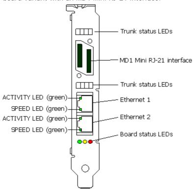
The following illustration shows the location of the LEDs on the CG 6565E board variant with MD1 RJ-45 interfaces:
