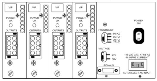
The power supply autoranges for global power standards and can be configured for local ring frequency standards to satisfy global deployment requirements.
