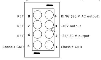
The mating connector is Positronics PLBO8M0050 with MC116N pins.
