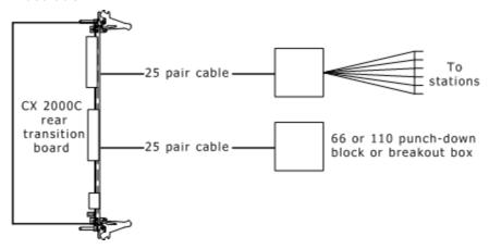
The RJ-21 connector on the cable must be the 180-degree design. The common 90 degree RJ-21 connector is not compatible with the CX 2000C board.
