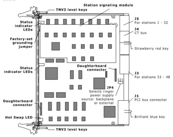
The following illustration shows where various components are located on the CX 2000C rear I/O transition board:
