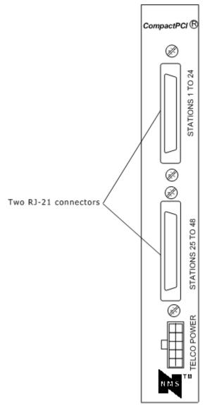
The connectors are each designed to accommodate a 25-pair cable. This cable is commonly wired to a punch-down block or break-out box. The telephones or other station devices are connected to the block or box through standard telephone wiring as shown in the following illustration:
