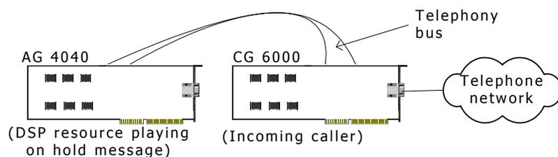
Using the PPX service, the application calls one function specifying both the location of the DSP resource (board number, local stream, and timeslot) and the location of the caller (board number, local stream, and timeslot). The PPX service determines the required telephony bus timeslots and makes the necessary switch connections.
