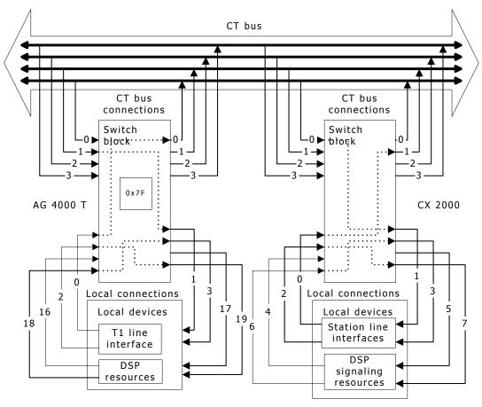
7. If either end hangs up, disconnect the call using the Natural Call Control service. Reconnect the AG 4000 board's DSP streams to the AG 4000 board's line interface streams.
