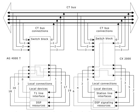
The following illustration shows the state of the switches in the system:
