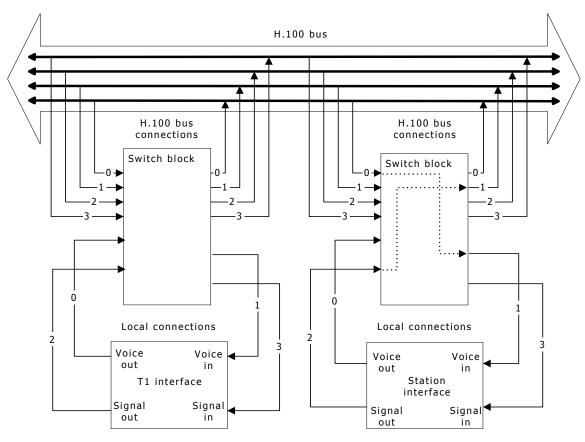
The following example code connects the incoming digital line's voice streams to the operator station's voice streams over the MVIP bus:
