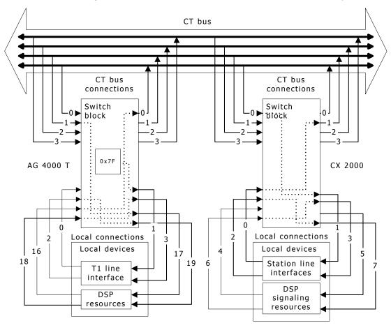
6. Connect the voice paths of the AG 4000 T1 line and the CX 2000 operator station so that the caller and the operator can carry on a conversation. To accomplish this task, connect the AG 4000 board's voice streams to the CX 2000 board's operator voice streams.
