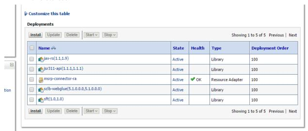
**Note:** If OCCAS was installed in **Production Mode**, click **Lock & Edit** and make the necessary changes. For the changes to take effect, click **Release Configuration**. When installed in **Development Mode**, this process is suppressed.
