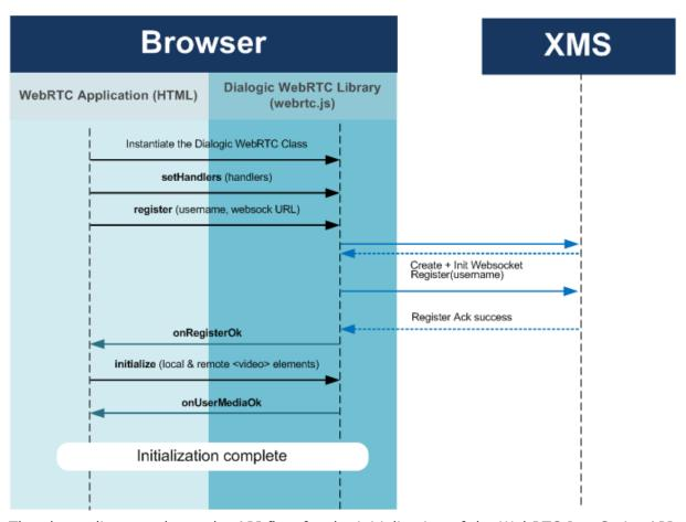
The above diagram shows the API flow for the initialization of the WebRTC JavaScript API library. The rest of the section details the code snippets corresponding to the flow.
