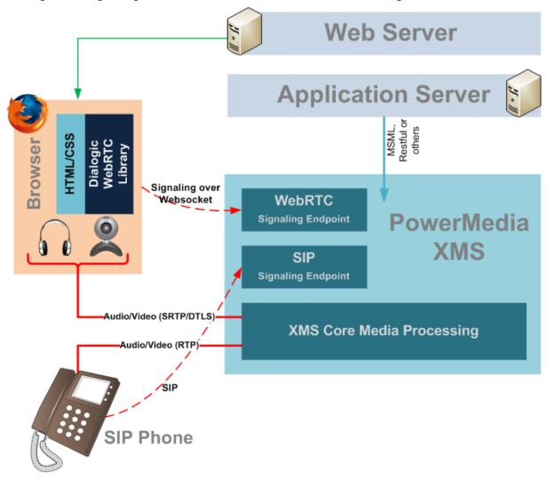
The Web Server hosts the Web Application, which embodies the front end of the WebRTC Application. As an example, this could be a retail website (like Amazon) which also provides users (of the website) with the ability to talk to their service representatives over an audiovisual channel in real time (for example, over WebRTC).
