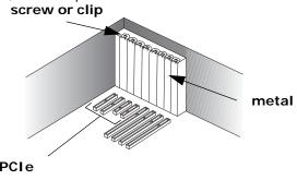
8. Firmly secure the Dialogic Blue Telephony Board with the screw or clip.
